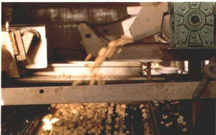
The mushroom is hand picked and in two hours is already processed. Most of the processing is done by machines that cut off roots, chop, wash, scald, and even classify by size. But a final selection must be done by hand to weed out defective or discoloured mushrooms.
