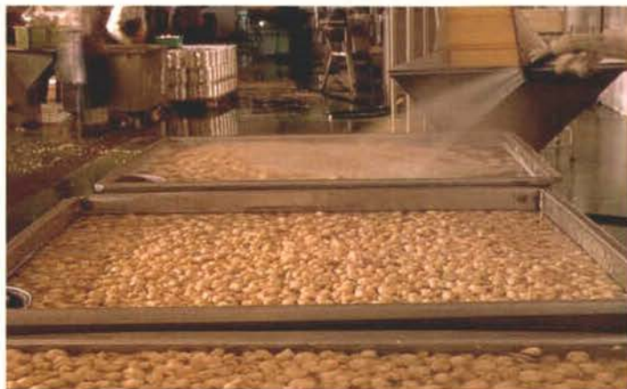
The mushroom is hand picked and in two hours is already processed. Most of the processing is done by machines that cut off roots, chop, wash, scald, and even classify by size. But a final selection must be done by hand to weed out defective or discoloured mushrooms.
