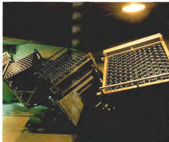
Mechanized system of bottle rotation "gyropalette"
